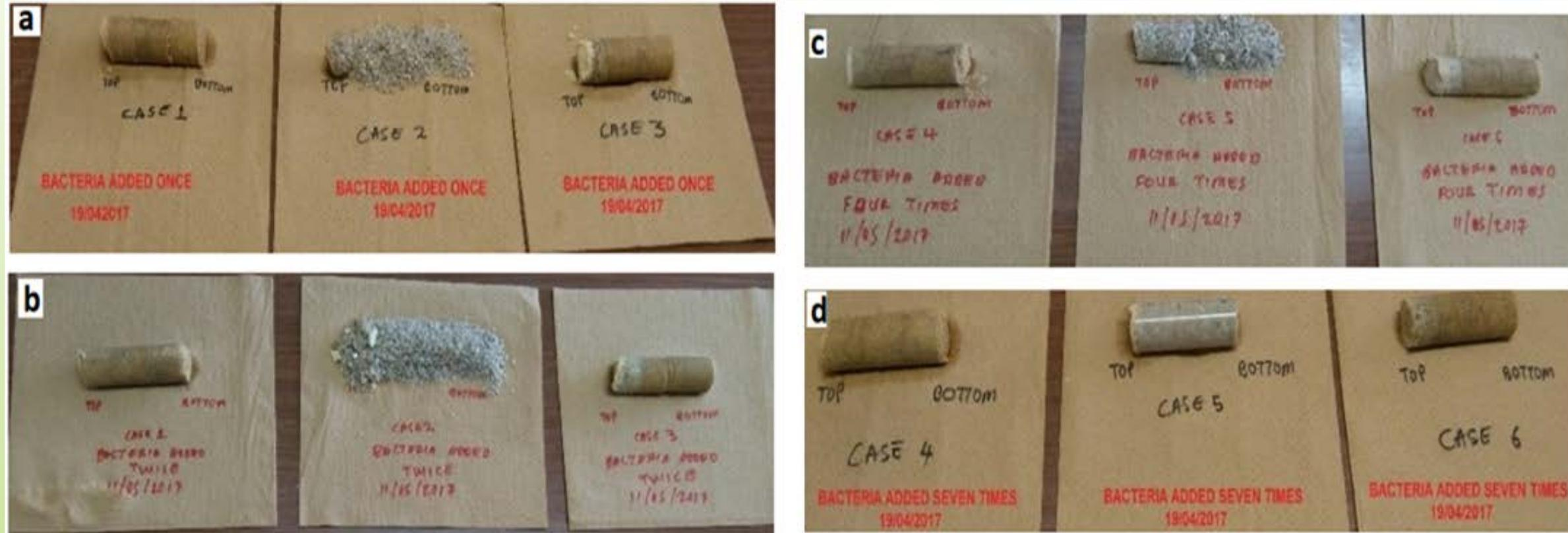
Pictorial images of the results of all syringe tests after 14 days while varying the bacterial injection interval to (a) one (b) two (c) four and (d) seven times. Left, fine sand; center, coarse sand; right, mixture of coarse and fine sand.
