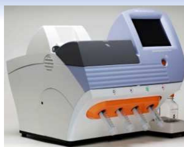
Soil DNA analyses using a next-generation sequencer
